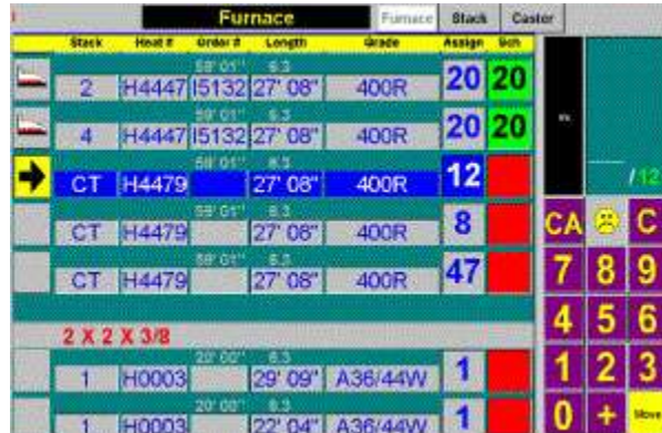
Fig. 15 – [PSC] Crane Operator's Touch Screen
