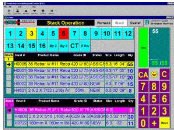
Fig. 16 - Crane operator Touch screen for billet movements from stack to stack
